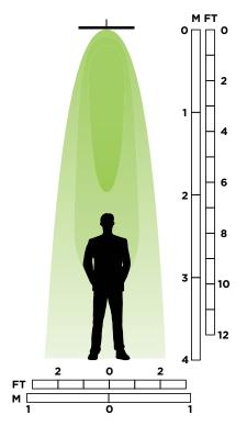
The loudest sound area is directly in front of the speaker panel at a distance of 1-2m. Sound levels outside the beam are reduced by over 90%.
